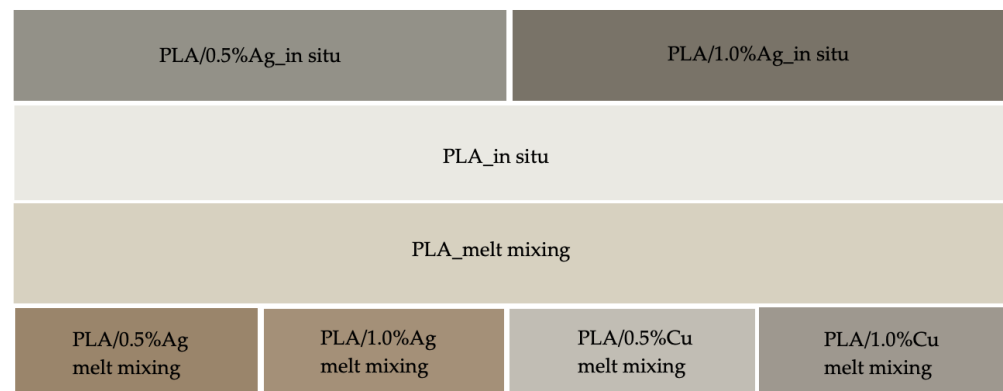
Figure 8. Color PLA samples and PLA nanocomposites, as recorded by the spectrophotometer.
